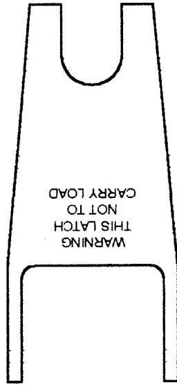
660522 USED ON ALL 1/2" CHAIN HOOKS JUNE 1999 THRU JUNE 2000 WE RECOMEND THAT YOU REPLACE THIS HOOK WITH P/N 615856 CLEVIS-TYPE HOOK
